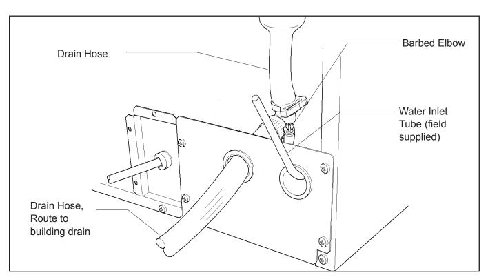
Back View, Gravity Drain Model
