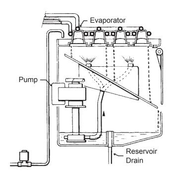
Freeze Cycle Water Schematic
