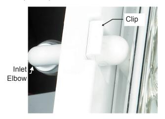
14. Pull clip up. Push inner elbow back and rotate it until it points straight up, then push it back through the hole in the back of the freezing compartment.
