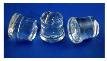
Normal cubes are tapered cylinders. If the cubes are ragged and mis-shaped, mineral scale must be removed from the ice making system
